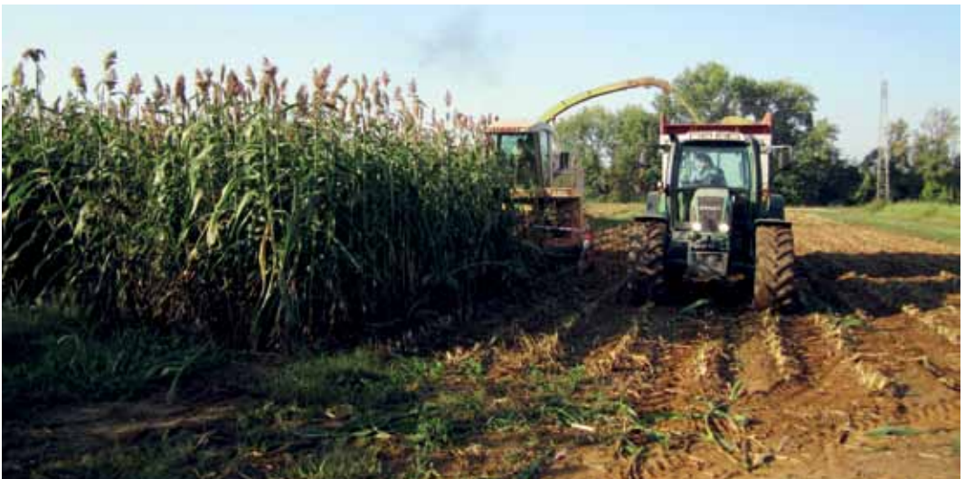
Figure 8: harvesting of sweet sorghum with mower-shredder-loader machine (source: CETA)
