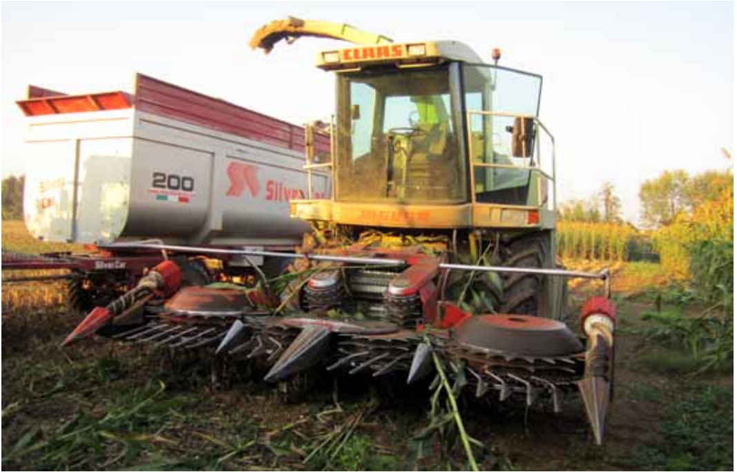
Figure 7: mower-shredder-loader machine (source: CETA)
