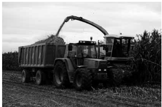
Figure 3: harvesting of sweet sorghum with mower-shredder-loader machine 30
