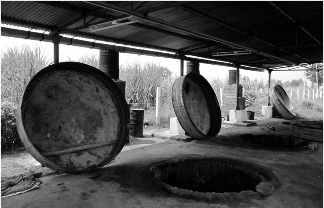
Figure 11: juice concentration unit at the DCU in Medak district, Andhra Pradesh (India) 61
